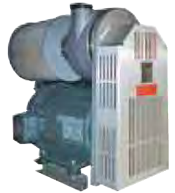
Centrifugal High Pressure Blower(s) in Dryer Section.
