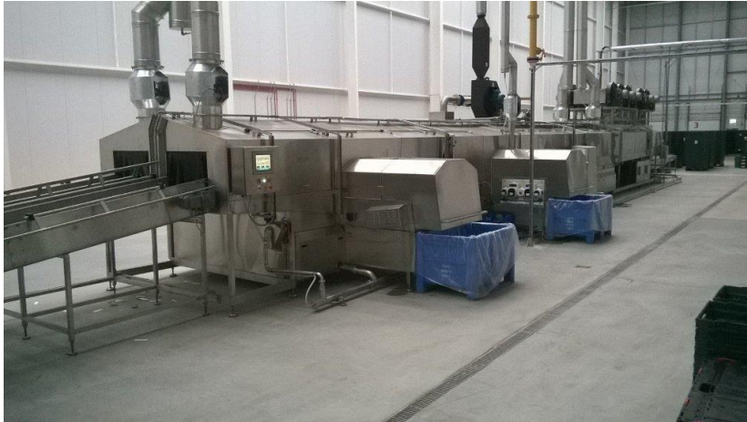
4000 TRAYS/HR PRE WASH / HOT WASH / HOT RINSE WITH HIGH PRESSURE LABEL REMOVAL AND AIR KNIVES
